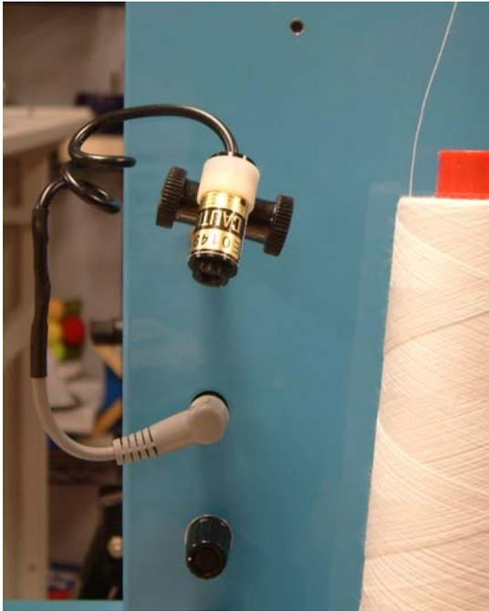
First, to mount the laser on the side, slide the laser onto the plastic stud and tighten the finger screws.
