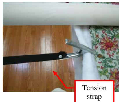
Check to see that your take up bar is all the way down to the lowest position. As you complete the quilt, you will have to raise this bar to have clearance between the quilt and the machine. You will do that by turning the crank at the end of the table. This system ensures that the quilt is raised equally on both ends.
